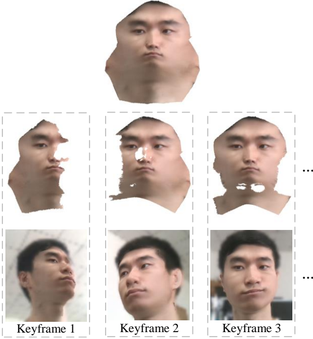
Fig. 3: M_i from each keyframe merged into the basic texture M . Mesh parameterization is only used to display the mesh in UV space, and is not necessary in our pipeline.
