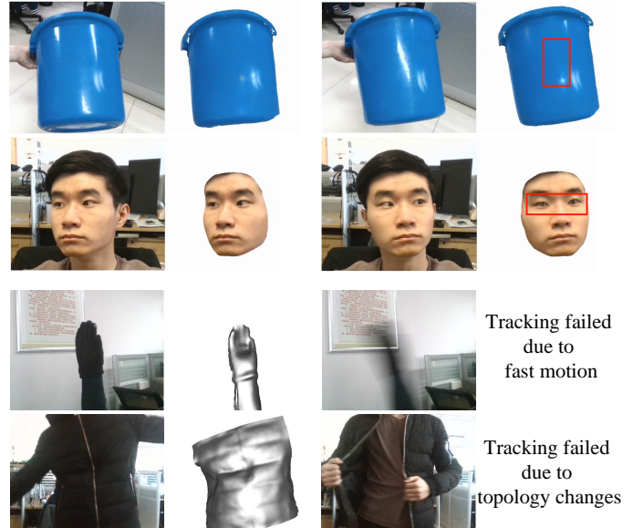
Fig. 13: Failure cases. Rows 1 and 2: texture reconstruction failure due to specular reflectance and eyeball movement, respectively; rows 3 and 4: motion tracking failure due to fast motion and topology changes, respectively.
