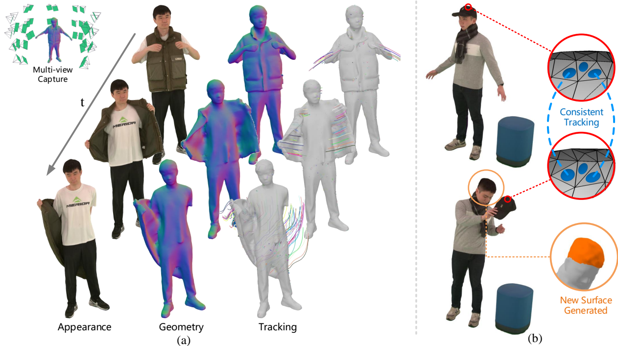
Figure 1. We propose GSTAR, a novel method that (a) enables photo-realistic rendering, surface reconstruction, and 3D tracking for dynamic scenes while handling topology changes. (b) GSTAR adapts to topology changes through two mechanisms: consistent tracking for stable surfaces (red circles) and dynamic surface generation for newly appearing geometry (orange circles).
