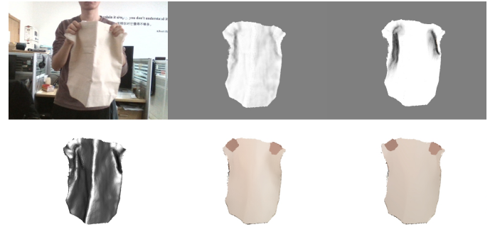
Fig. 10. Comparison with AO reconstruction. Left: input color image and reconstructed geometry; middle: percentage of light not occluded and reconstructed albedo in AO reconstruction; right: our percentage of light not occluded and our albedo. (Gray scale [0, 255] corresponds to percentage [0, 100%])
